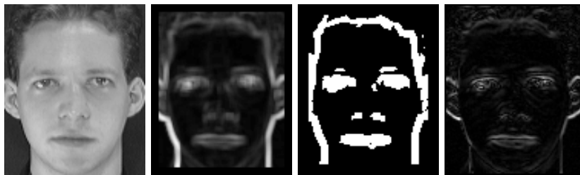
Fig. 1. Preprocessing example. From left to right: original image, local variance image, thresholded variance image with selected pixels in white, and gradient image.
